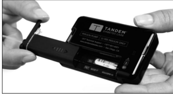
300-unit Insulin Cartridge being inserted into Pump
