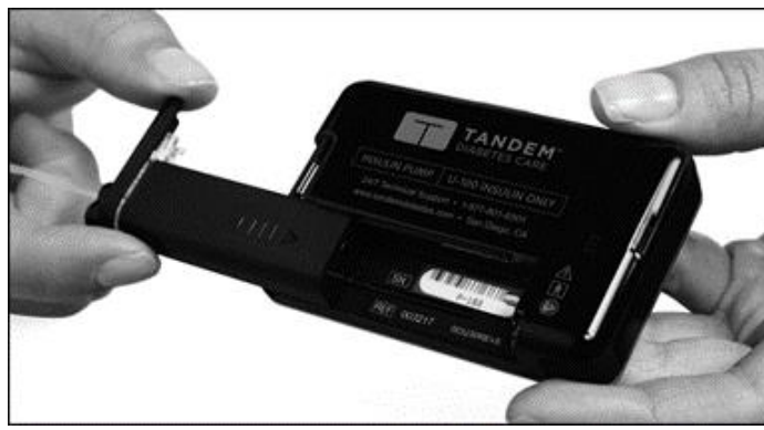
300-unit Insulin Cartridge being inserted into Pump
